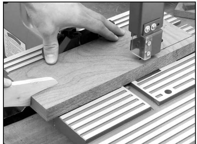
Figure 30. Ripping with a push stick.
